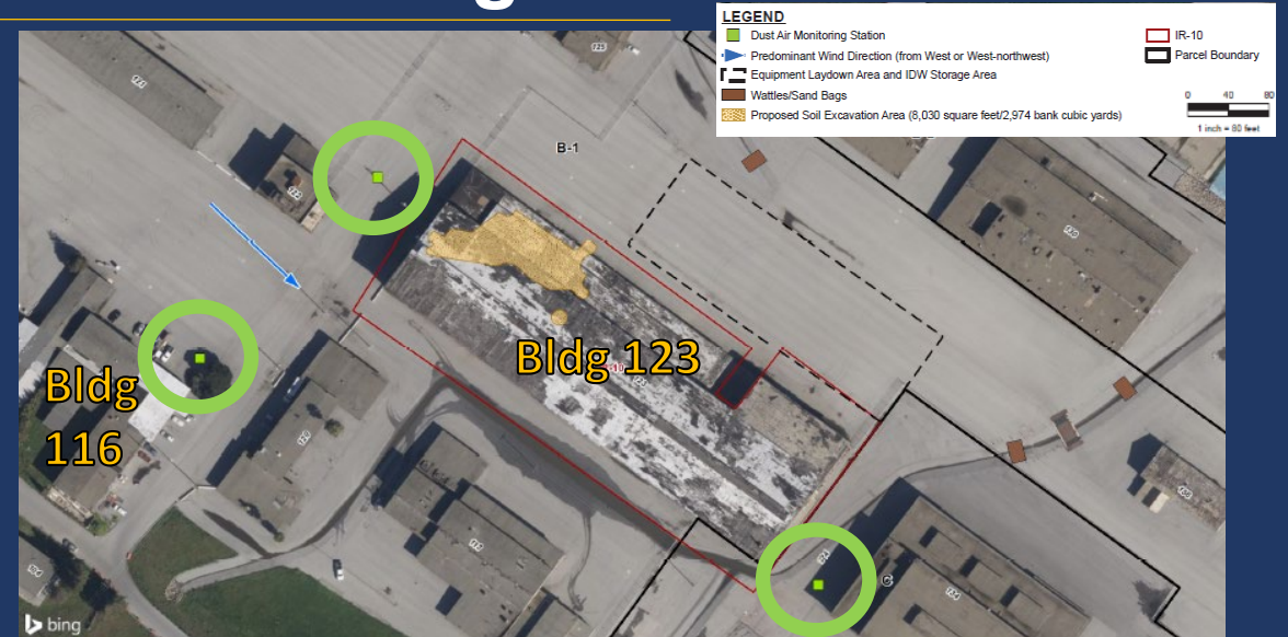
Location of air monitoring stations during Building 123 demolition, approximately 10 feet from each respective building
